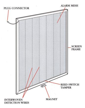
The concept of the **SECURITY SCREEN** is really quite simple. Your existing frame, or new custom made frame, is screened with special alarm mesh which has interwoven detection wires every four inches.
